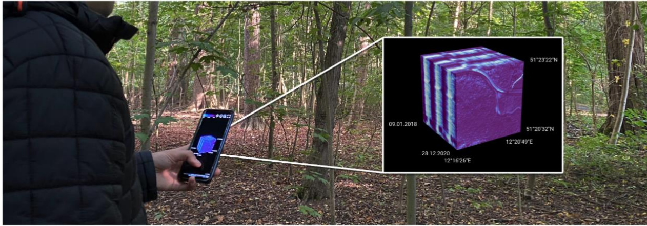
Figure 1: A user with the Lexcube application on her smartphone, visualizing a data set of the protected area “Auwald forest”, Leipzig, Germany, while walking through it. The spatiotemporal data visualization shows longitude by latitude on the cube front face, and latitude/longitude by time on the side faces. This data cube view enables visual comprehension of temporal patterns and trends. Here, the kNDVI spectral index (Kernel Normalized Difference Vegetation Index) based on satellite imagery from a commercial data provider is on display.
